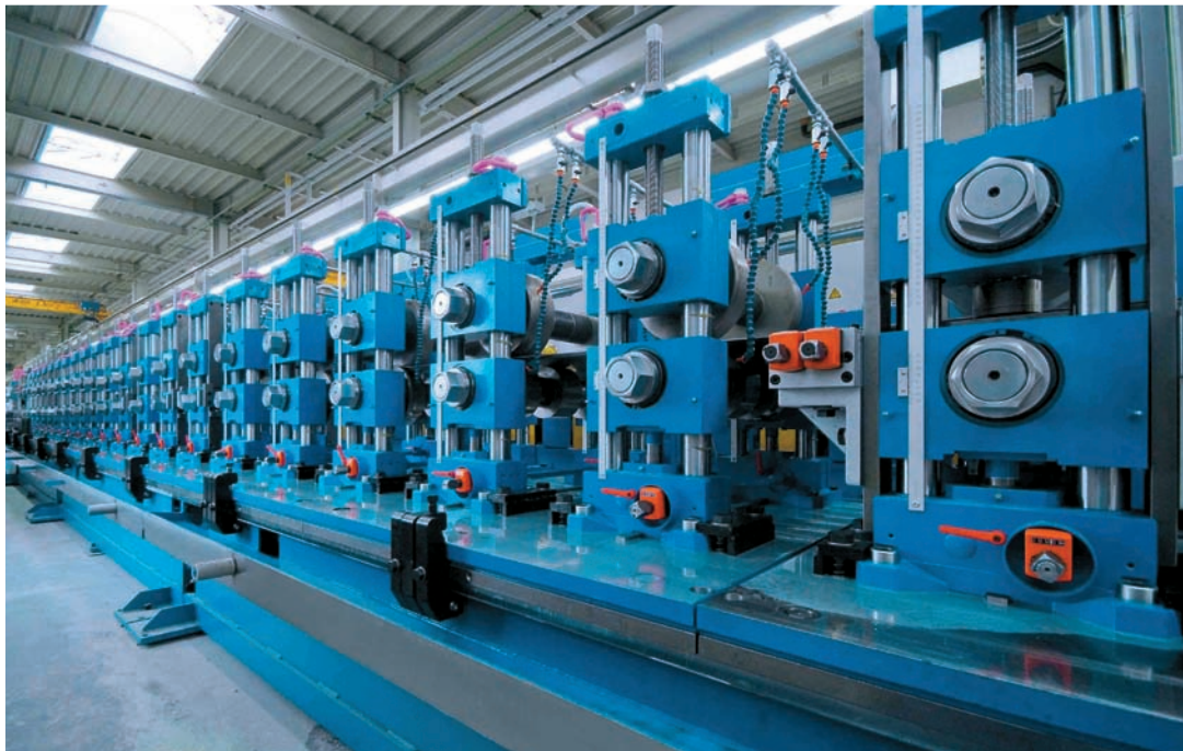
The Dreistern roll former at Metalsa's production for their "Light Vehicles" business unit.
