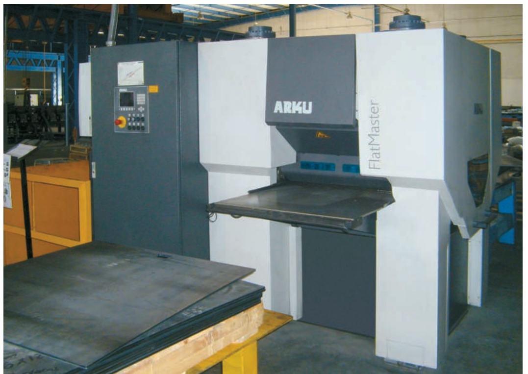
All sheet metal parts at DIMET go through the FlatMaster 50 to meet high-quality standards and to save costs during subsequent welding and material procurement
